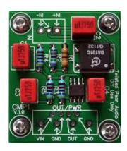
For this board, R1 is the level resistor (like  $RS_{<Z>}$  is on the S/PDIF-4 Input Board) and R2 is the termination resistor (like  $R_{<Z>}$  is on the S/PDIF-4 Input Board). For the correct values of these resistors see the table below.
