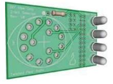
On the switch module, the 4 pins (<u>on switch module: EXT\_IO, 6</u>) you need to use are conveniently marked with a rectangle on the rear of the board. Also four 2-pin connectors are located at the rear of the board (<u>on switch module: LEDs, 5</u>) in a convenient 0.1"x0.1" pitch grid, to simplify the connection to off-board LEDs. The individual connectors are numbered from 1 to 4 to indicate which connector corresponds to which LED.
