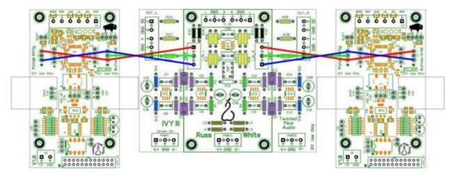
Bridging the outputs increases the signal that goes into the I/V stage. Depending on the I/V stage it may be required to correct the gain of the I/V stage, as described in the next section.
